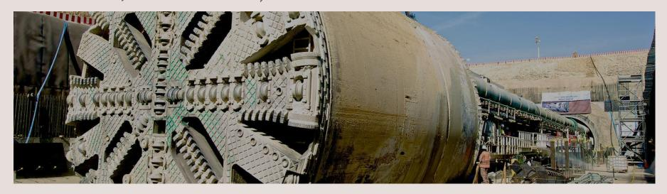
Line 3 and 5 of Riyadh underground are 41 km and 12.9 km long and they are bored by a TBM tunnel (EPB). Along the TBM tunnel there are some underground stations and evacuation or ventilation shafts with connecting galleries.
